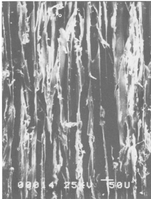
FIG. 7—SEM tangential section of Idaho pine ( Pinus monticola ).
